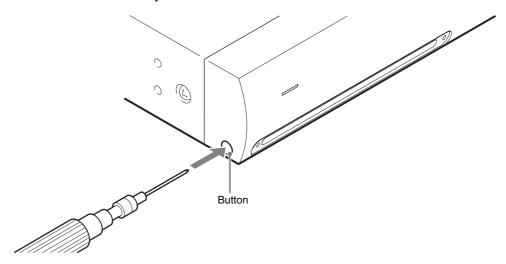
The end of the air filter is slightly ejected.
